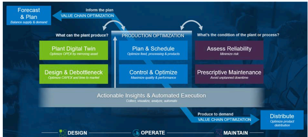
Figure 2: Asset Optimization Digital Reference Architecture from AspenTech. This is a blueprint both for customers and for AspenTech innovation R&D. This digital reference architecture aligns with the breadth of AspenTech’s digital twin solution (pictured on page 4). The left-hand boxes in the image above represent the plant digital twin, the center boxes represent the operational excellence digital twin and the right-hand boxes correspond to the operational integrity digital twin.
